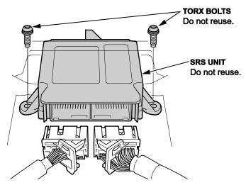
7. Write down the new SRS unit ID (serial number) on the RO, then install the new SRS unit using the new Torx bolts.
