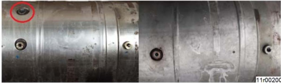
Figure 1, Obsolete SCR Catalyst (left) and New SCR Catalyst (right)
