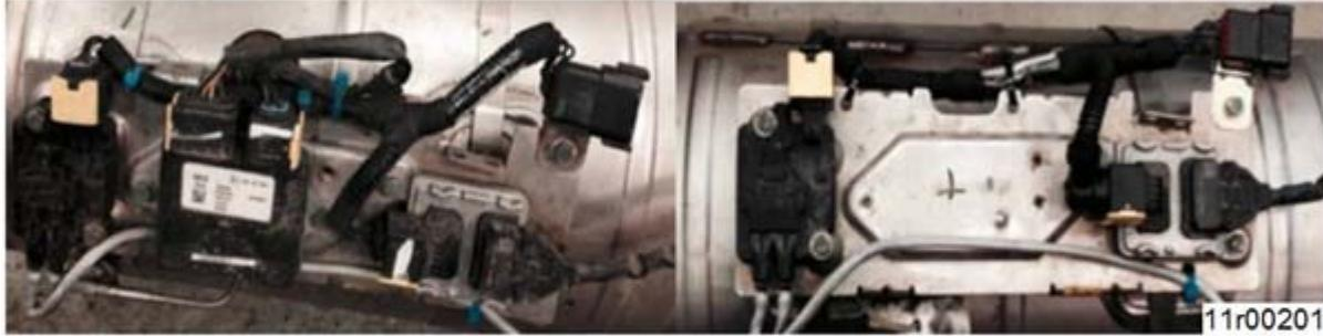
Figure 2, Three Sensor Aftertreatment SCR Wiring Harness (left) and Two Sensor Aftertreatment SCR Wiring Harness(right)
