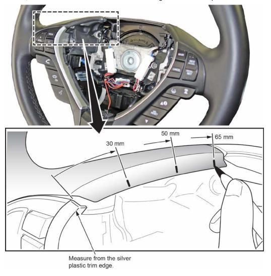
7. Measure 6 mm from the top edge of the spoke down towards the bottom of the leather material, and scribe marks at 30 mm, 50 mm, and 65 mm. Do this on both the right and left side spokes.
