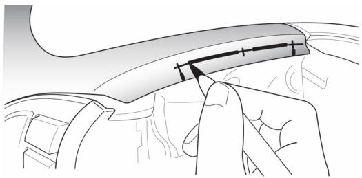
9. Using a new flat razor blade, cut out the rectangle to remove the excess leather material from the steering wheel on both the right and left side spokes.
