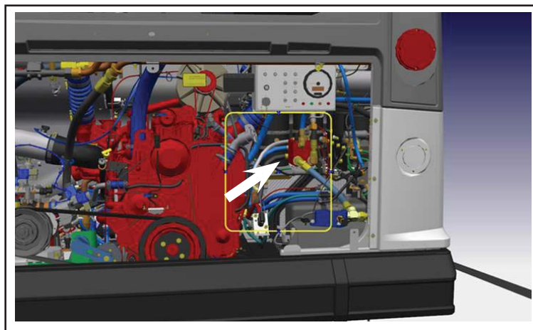
Figure 1 - Location of the Hydraulic Fan Control Manifold
