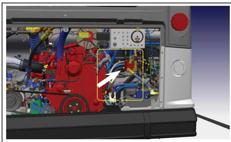
Figure 1 - Location of the Hydraulic Fan Control Manifold
