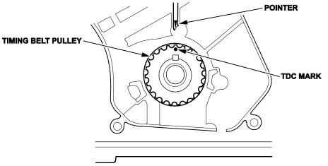
• Align the TDC marks on the camshaft pulleys with the pointers on the back covers.
