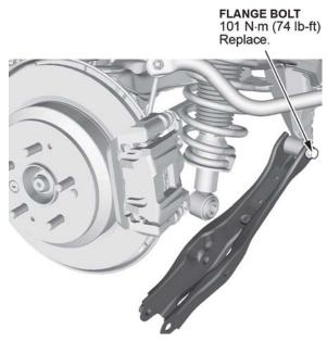
19. Position a floor jack under the lower arm. Then gradually raise the arm into place and loosely install new flange bolts.
