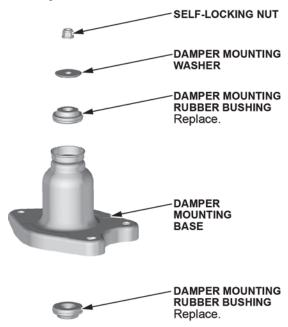
12. Assemble with the new damper unit and damper mounting rubber bushings as shown below. Do not install the mounting washer and self-locking nut at this time.
