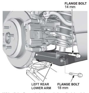
20. With all the flange bolts loosely installed, load the suspension with the vehicle's weight.
