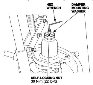
17. Install the damper assembly and loosely install the new upper flange bolts.
