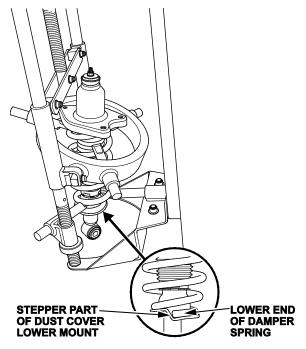
15. Align the angle of the bolt hole on the damper mounting base with the bottom of the damper unit.
