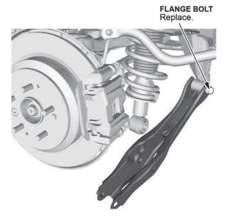
7. Remove the upper damper mount flange bolts and remove the damper assembly. **DAMPER ASSEMBLY**
