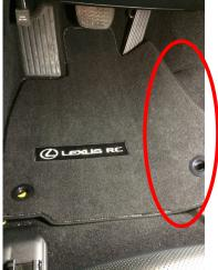
The edge of the mat does not fit in the vehicle correctly.
