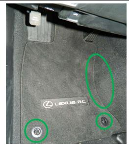
The mat should fit around the transmission tunnel as shown.
