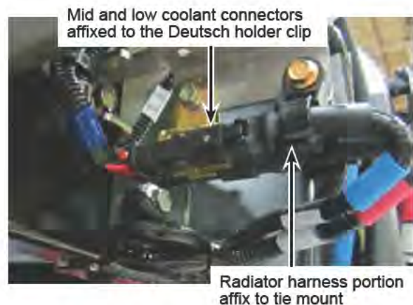
Figure 4 - Installation of Harnesses to the Support Bracket
