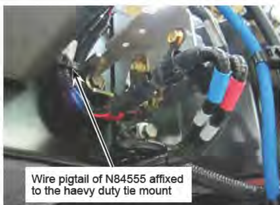
Figure 4 - Installation of Harnesses to the Support Bracket
