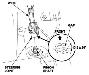
26. Align the bolt hole on the steering joint with the groove around the pinion shaft, then loosely install the steering joint bolt. Be sure the joint bolt is secure in the pinion shaft groove.
