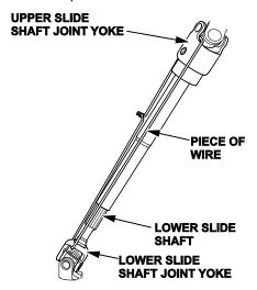
11. Remove the steering joint bolt, then disconnect the steering joint from the pinion shaft.
