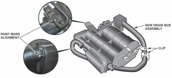
7. Install the new drain box bracket and new retainer as shown.
