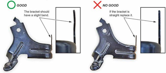
3. Install the new bracket and torque the nut to 9.4 N·m (6.9 lb-ft), Then install the harness to the bracket.
