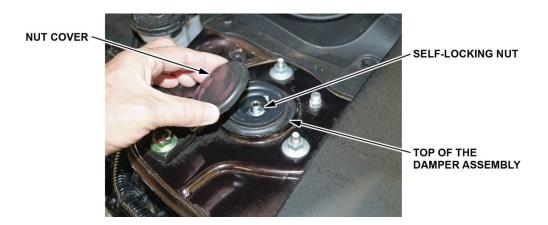
2. Torque the two self-locking nuts located at the top of the front damper/spring assemblies using a 6 mm hex wrench, a 17 mm socket, a strut nut adapter, and a torque wrench set to **70 N-m (52 ft-lb)**.
