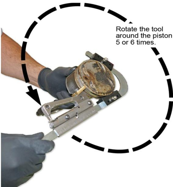
7. Remove the piston groove cleaning tool and clean off the carbon from the tool bit.
