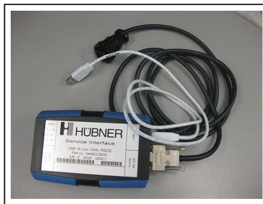
Figure 2 - Hübner Service Interface (Part N° N8900610)
