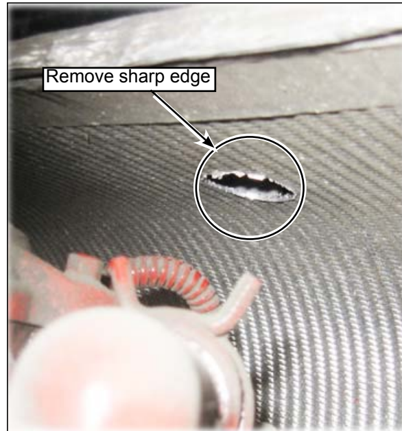
Figure 3 - Remove Sharp Edges and Clean with Isopropyl Alcohol
