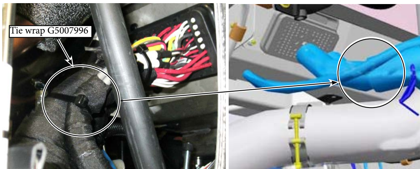
Figure 10 - Attach Wire Kit
