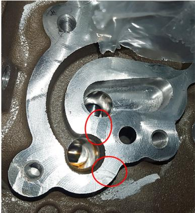
d) The oil filter adapter may have a defect leaking in the aluminum casting on an LFX engine with cartridge style filter. See picture below.
