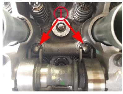
b) If soft or spongy SHLAS are found, carefully remove the affected head and inspect the oil passage below the head gasket for debris.
