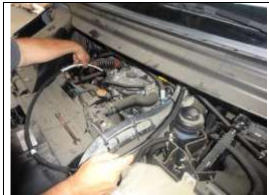
Figure 10 – A/T Shift Cable Removal
