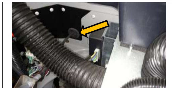
Figure 7 – Rubber Grommet at the Engine Wall
