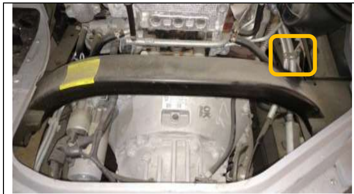
Figure 5 – Mounting Bracket at Passenger Frame Rail
