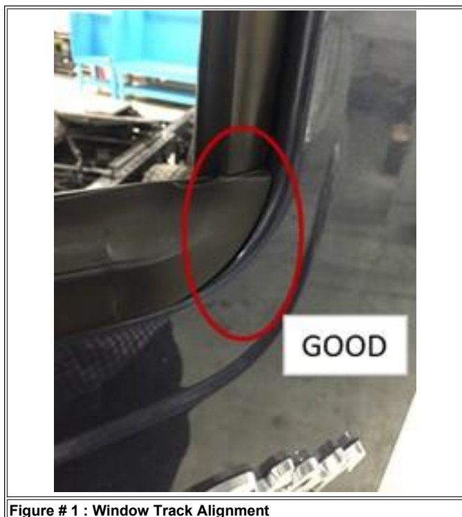
Figure # 1 : Window Track Alignment
