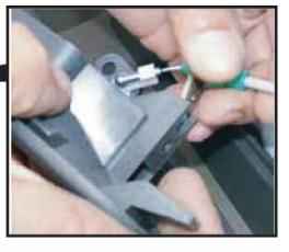
3. Separate the cable end from the clip (snap).
