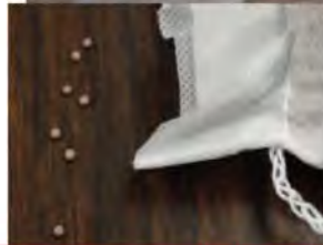
Mohawk Loose stitch allowed desiccant to escape
