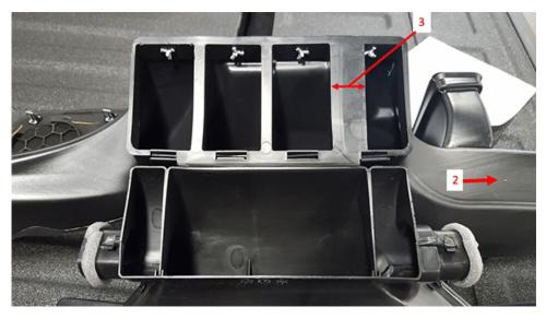
3. Measure over 20 mm (.787 inches) (4) and mark the air distributor duct, as shown below. Using a sharp utility knife, cut out the portion of the deflector that is marked.
