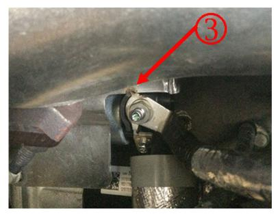
3. Inspect for any high resistance and/or loose connections at both the battery fuse block and the positive or negative battery cables. If no loose connections are found, perform a loaded voltage drop test on the positive and negative battery cables, as well as the positive battery cable between the battery "+" post and the Battery Fuse Block (4), as shown below.
