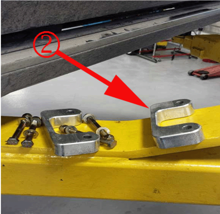
2. Aftermarket lift kit blocks removed from a truck
