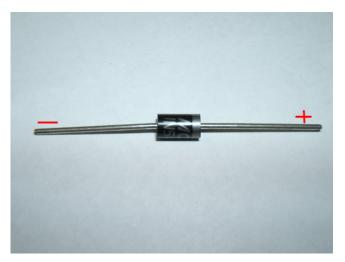
Install a diode, P/N 12112422, across the coil of the solenoid. It is important that the striped end of the diode be connected to the positive terminal of the coil and the other end of the diode be connected to ground.
