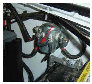
Important: Be sure to insulate the diode with heat shrink tubing before installing as shown in the picture above.
