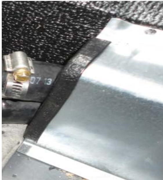
Figure 8, Installation of edge guard on metal cover
