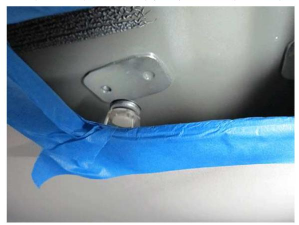
8. Coat the backside of the metal plates with the adhesive and install the plates using the alignment marks created in step #4. Tape the plates into position
