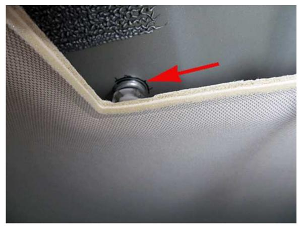
4. Using a paint pen or marker, mark the location on the inside of the roof panel where the magnets attach.
