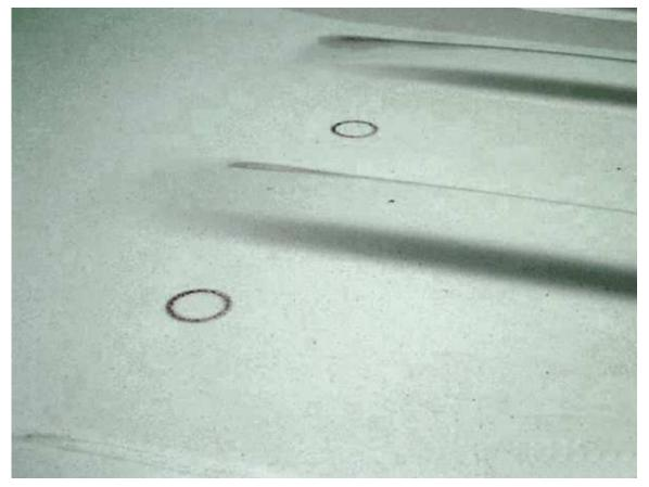
Some customers may comment that two dark circles of paint discoloration have formed in the center of the exterior roof panel. This condition is most noticeable on light colored vehicles.
