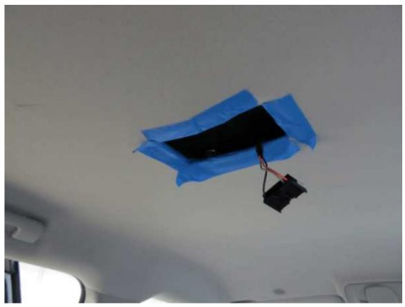
3. Protect the headliner with masking tape and cover the interior to protect from glue contamination.
