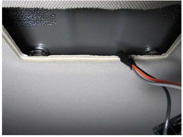
2. Remove the second row courtesy lamp. Refer to Courtesy Lamp Replacement in SI.
