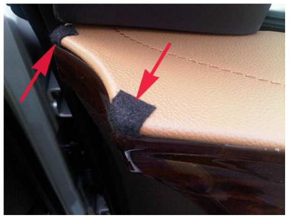
Two pieces of adhesive backed flocking material (black felt) are installed on the front side door interior trim panels as shown. This material is installed to protect the door panels during the build process.
