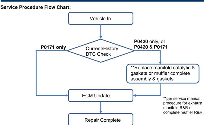
**NOTE:** If significant honeycomb material has broken apart from the exhaust manifold catalyst or muffler assembly, blow out with compressed air to remove any residual catalyst material from the exhaust tube and underfloor catalyst.
