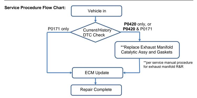
**NOTE:** If significant honeycomb material has broken apart from the exhaust manifold catalyst, blow out any residual catalyst material from the exhaust tube and underfloor catalyst.
