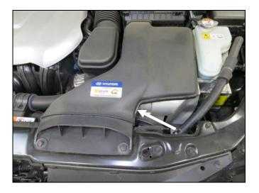
6. Remove the air intake hose and air cleaner assembly.
