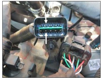
9. Disconnect the extension motor wire connector from the temperature sensor at the transaxle.
