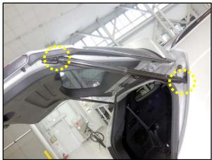
6. Check if the wire grommet (G) is securely installed. Reinstall the grommet (G) if necessary.
