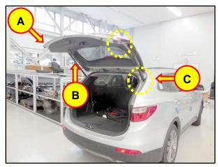
2. Remove the tailgate lifter mounting bolts (C).
