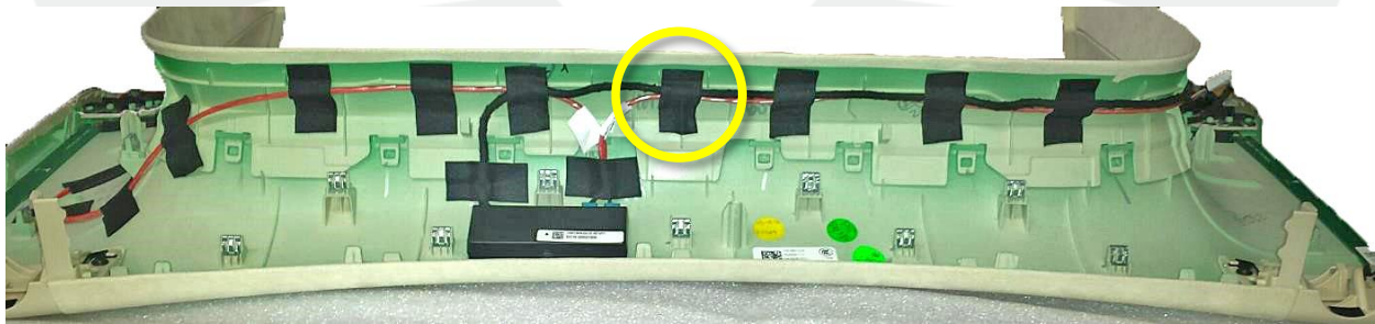
✓ Figure 1 (Harnesses bundled and secured with black polyester electrical tape)
