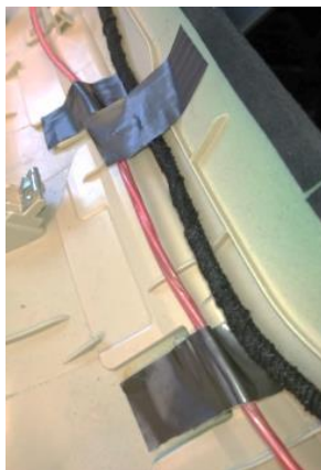
✗ Figure 3 (Harnesses secured with duct tape)
