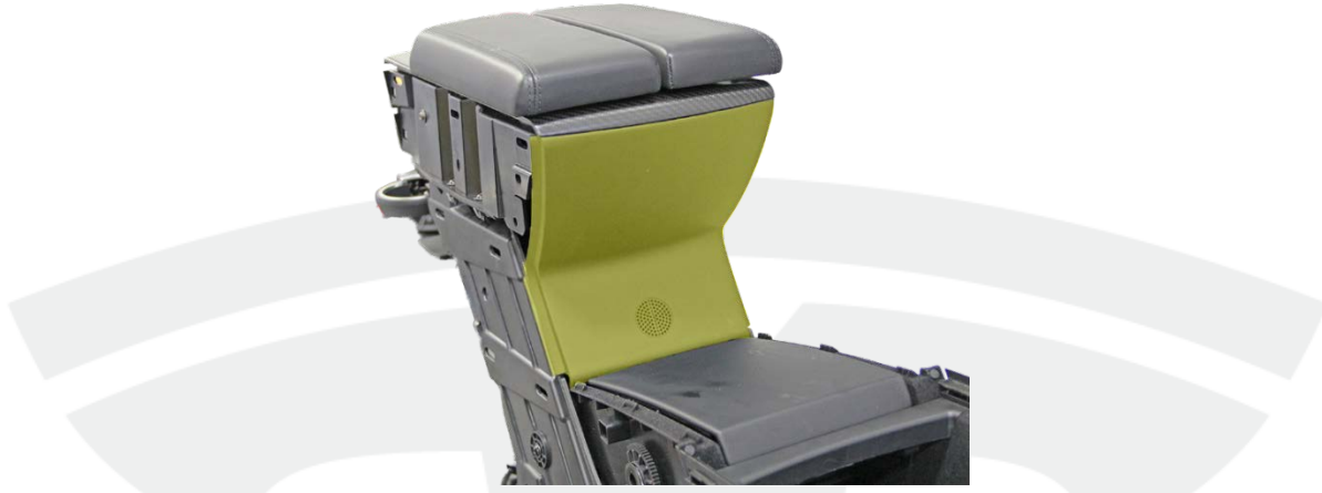
Figure 24 (Front closeout panel highlighted)
