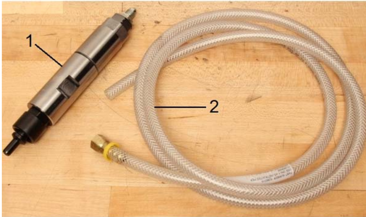
Figure 1, Fuel Pump Performance Test Kit, Part Number 5299721.
