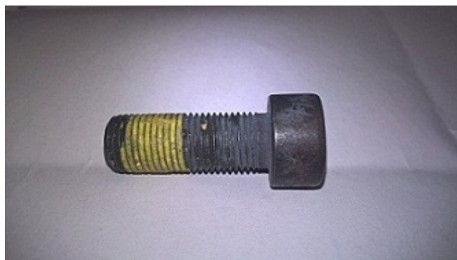
Figure 7. New generation bolt (part number WHT007991 (M10x1x27))
