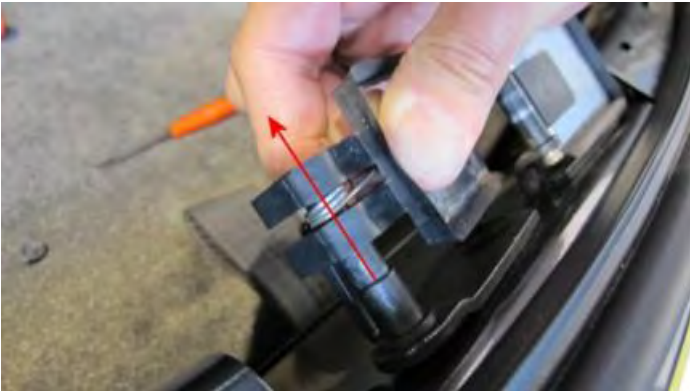
Figure 13 Slid door and spring off the bearing pin discard the original spring (see Figure 13)
