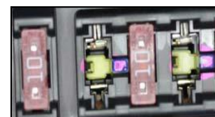
Loose Fit Between Fuse terminals
