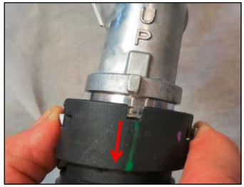
7. Press the tab on the bottom side of the coolant temperature sensor connector and disconnect the connector.
