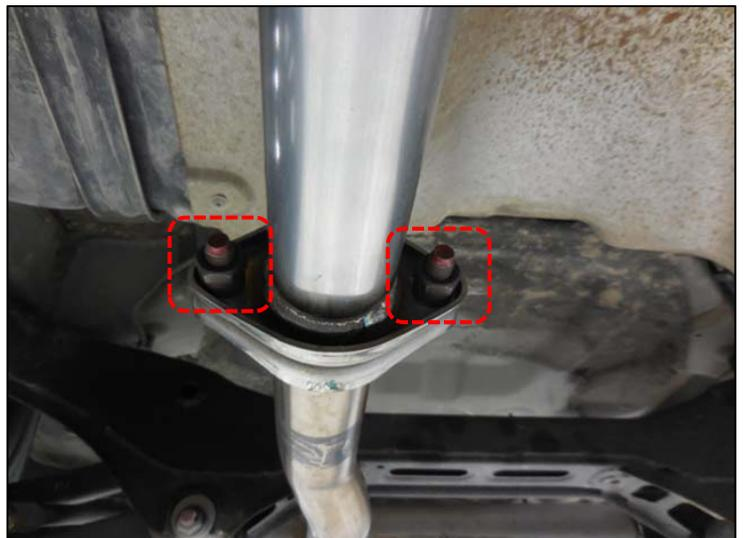
12. After making sure that the two cut ends of the pipes are butted together inside the clamp:
