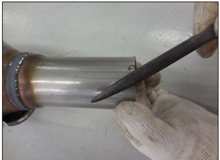
5. Locate the front dent (H) and rear dent (G) of the new replacement campaign center muffler pipe for cutting at rear dent point (G).
