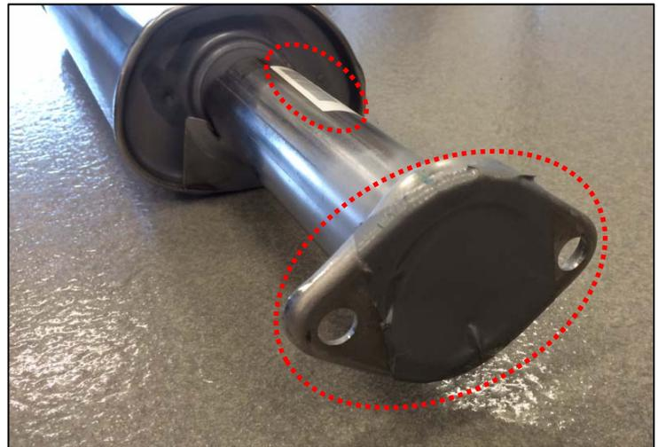
7. Reuse the front flange gasket and install the catalyst (F), then temporarily hand tighten the flange nuts.
