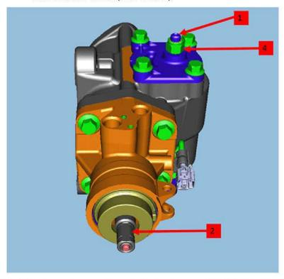
13. Tighten the steering gear pitman shaft lash adjuster nut (4) to 75-85Nm (55-63 lb ft).
