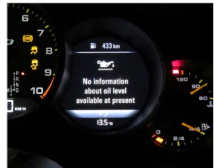
Oil level information in the multi-function display
