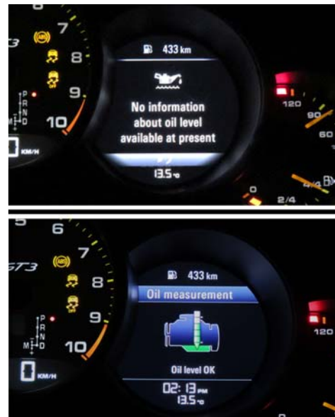
Oil level information in the multi-function display
