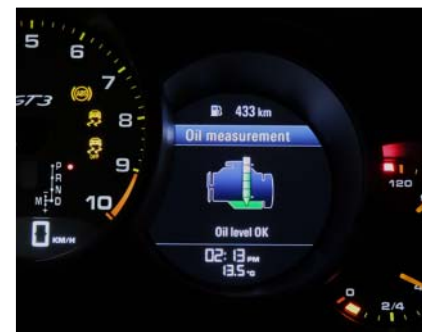
Oil level display on the multi-function display
