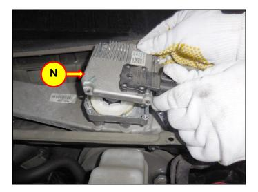
11. Use a T20 Torx screwdriver and remove the four Torx head screws (M) from the wiper motor cover.
