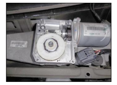
13. Place the new seal (O) on the motor.
