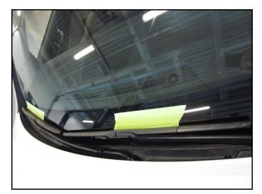
3. Place a piece of tape on the windshield in parallel to each wiper blade to mark the position of the wiper arms.
