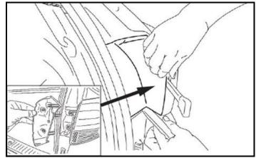
7 Remove the two (2) 10mm bolts securing the passenger side tail light. Dislodge the tail light from the vehicle.
