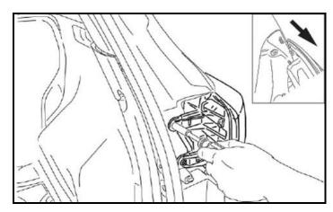
8. Disconnect the passenger side tail light Tow Module Harness 6-Pin Female Connector from the tail light, then remove the passenger side tail light from the vehicle.
