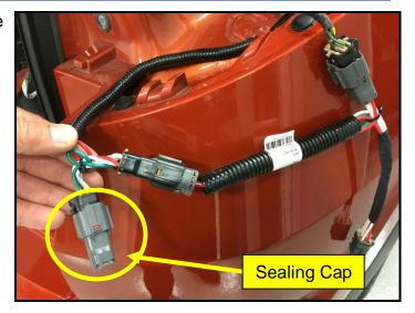
13. Bundle the Tow Module Harness connector with Sealing Cap and the Repair T-Harness as shown.
