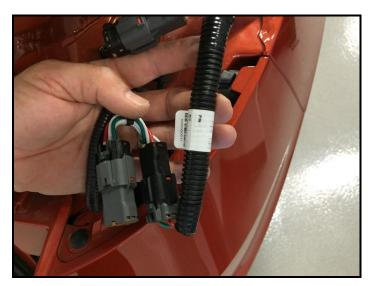
14. Use 2 foam tapes to completely wrap over the Repair T-Harness corrugated tubing, Tow Module Harness connector and Sealing Cap as shown.
