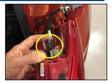
19. Before reinstalling the passenger side tail light, bundle the Repair T-Harness close to the tail light as shown.
