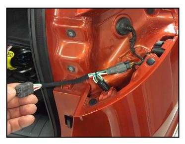
17. Attach one (1) foam tape to the passenger side Vehicle Harness 6-Pin Female Connector and the Repair T-Harness 6-Pin Male Connector as shown.
