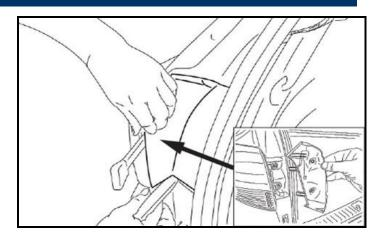
4. Remove the two (2) 10mm bolts securing the driver side tail light. Dislodge the tail light from the vehicle.
