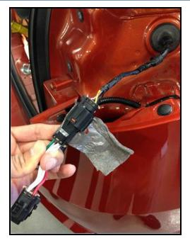
Attach the passenger side Vehicle Harness
