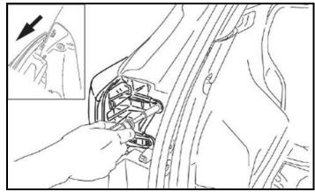
Disconnect the driver side tail light Tow Module Harness 6-pin Female connector from the tail light, then remove the driver side tail light from the vehicle.
