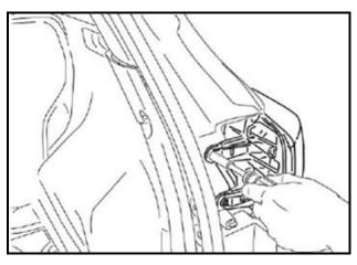
22. Reinstall the black plastic cover making sure all four (4) clips are fully engaged.
