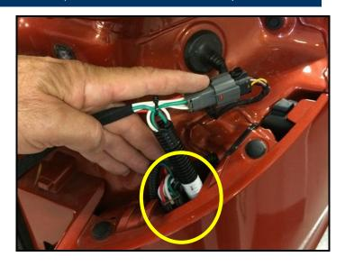
16. The Repair T-Harness should appear as shown.
