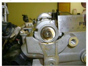
**Notice:** Each of the procedures above may not detect a small movement in the reluctor, it may be necessary to compare to a known good engine if in doubt. Also note that the cam cover gasket surface does not line up with the same face/slot on the intake and exhaust reluctor.
