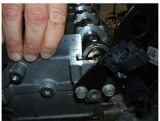
To check the Intake Cam reluctor position LE5 ONLY:
