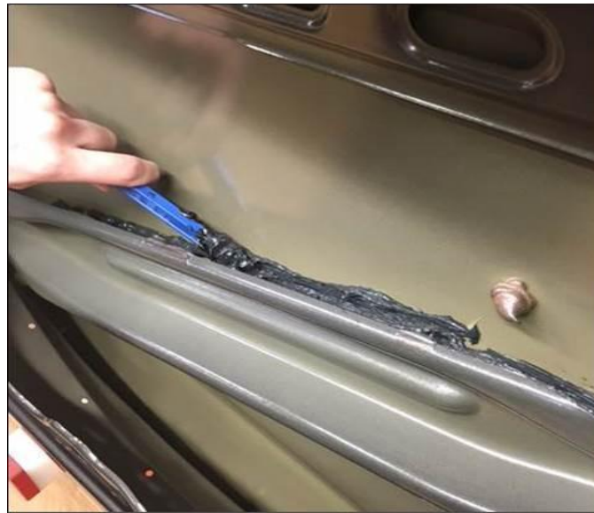
Fig. 2 Use Trim Stick To Force Into Space
