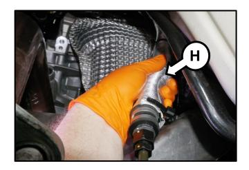
9. Inspect the power steering hose routing to make sure there is a minimum of 0.4" (10mm) of clearance between the heat shield and the exhaust manifold.
