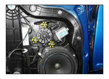
10. Disconnect the wire harness connector from the window motor.
