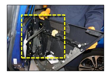
9. Remove three (3) screws securing the window motor to the door module.
