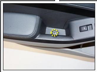
6. Dislodge the bottom portion of the door panel using a non-marring trim panel removal tool.
