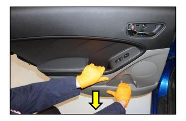
8. Disconnect the door handle cables and the power window switch connector to remove the door panel.
