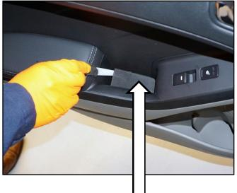
5. Remove one screw from the coin pocket area of the door panel.
